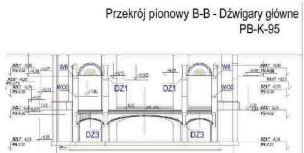
Fig. 73. Main girders for ground level floor, A3.
