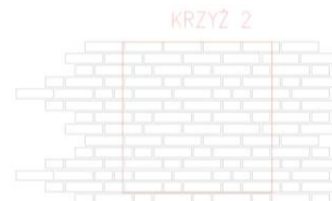
Fig. 39a. Second bricks arrangement in wall – named as “cross 2”
